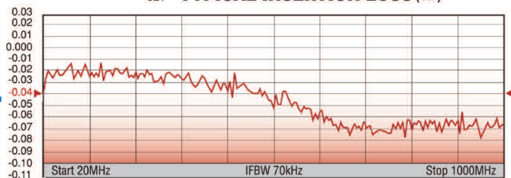
S21 TYPICAL INSERTION LOSS (dB)
