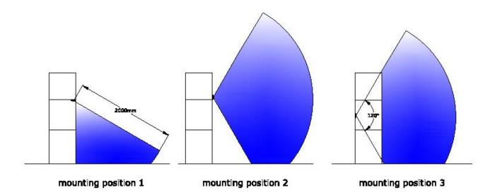
Note: this picture shows that the pir sensor can be installed in different locations, and then the effective zone is different. You may choose correct mounting location according to your purpose.
