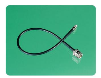
40 cm coaxial cable (RG 58) with one FME-connector (female) at one end and one N-connector (female) at the other end. The coaxial cable applied is a special PROCOM design. It has the lowest possible loss for an RG 58 coaxial cable (below 0.5 dB/m at 900 MHz) and a very exact 50  $\Omega$  impedance.
