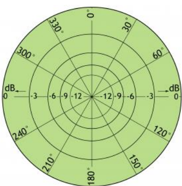
TYPICAL RADIATION PATTERN (H-PLANE)
