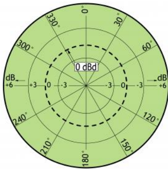
TYPICAL RADIATION PATTERN (H-PLANE)
