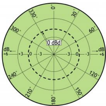
TYPICAL RADIATION PATTERN (H-PLANE)
