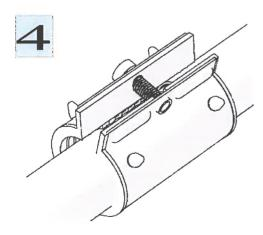
Close the grounding clamp and tighten the screw.
