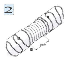
Strip off the jacket of the coaxial cable approx. 26-28 mm using the cutter knife.
