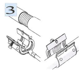
Insert the coaxial cable in the open grounding clamp.
