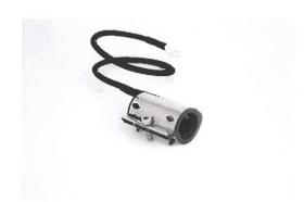
The grounding clamp for 10 mm coax cables such as Ecoflex 10, Aircom Premium etc. is used to eliminate potential differences (voltages) between the coax cable and the earth potential, which can occur, for example, during a thunderstorm. The grounding clamp has a solid stainless steel housing with a hinge and thus a compact structure. Installation is fast and easy because there are no loose parts and the earthing clamp can be closed with just one screw. No extra taping is needed.
