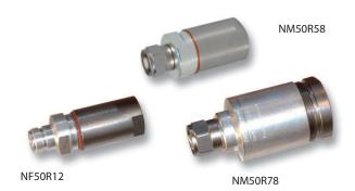
The connectors are designed according the standard interfaces as N or DIN 7-16. Contact components are silver plated to minimize insertion loss; mechanical parts are nickel plated for heavy-duty handling and best corrosion resistance. The special quick trimming tool make installation very easy and cost effective in time.
