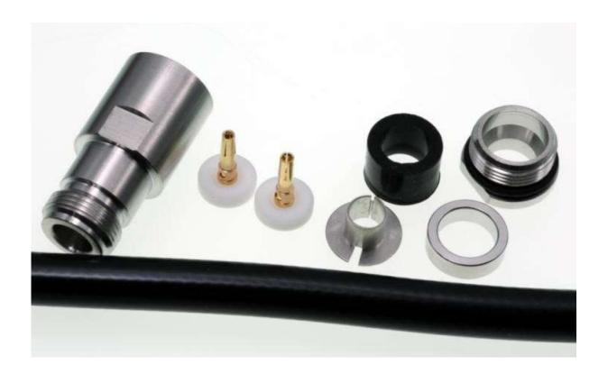
N 23 ECO-TA is delivered with 2 center pins. The difference is to be seen between the drilled holes for the cables and the holes for the solder contact. The center pin with the bigger solder contact is suitable for Ultraflex 10, Ecoflex 10, H 2010, Calorix 10 and similar cables. Please use the second contact for all the other cables of the list.
