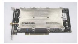
The PCI card plugs into an available slot of an IBM-compatible PC. Several receivers (as many as there are free PCI slots available) can be controlled by a single PC - an ideal solution for highperformance multi-channel automatic monitoring systems.
