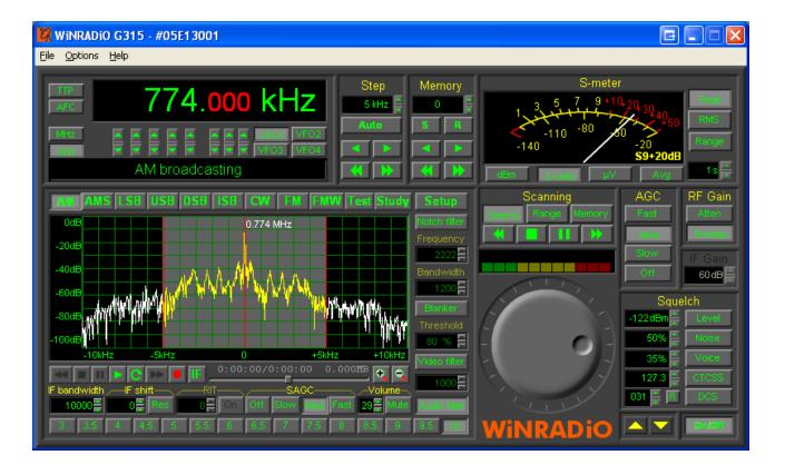
There are numerous demodulation modes, continuously variable IF bandwidth 1 Hz to 15 kHz (in 1 Hz increments), a 20 kHz wide real-time spectrum analyzer with 16 Hz resolution, noise blanker and notch filter. There is also an integrated recorder, making it possible to instantly record and playback the received signal.
